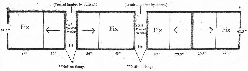
\*\*Vinyl mull cap piece provided by manufacturer and installed by contractor.
